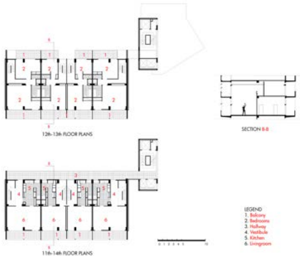
Figure 3. Plan views and section of the duplex, levels 11-14, Sabena Towers. Drawing by Manlio Michieletto.
