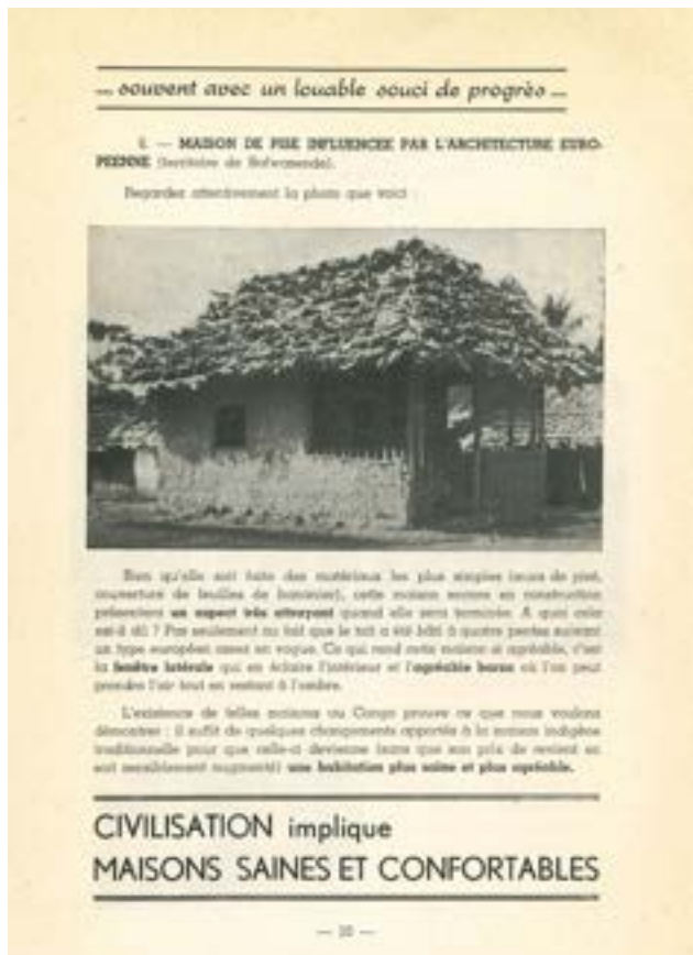
Figure 8. À chacun sa maison , House 6, 'House of rammed earth influenced by European architecture (Bafwasende territory)', 10.
