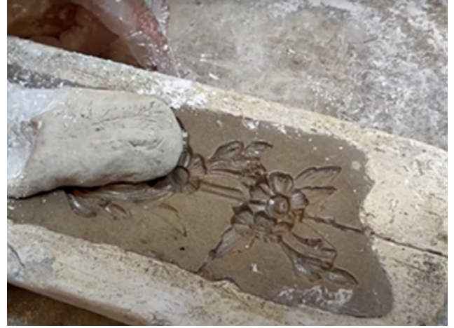
Figure 2. Placing the carton-pierre molding dough into the mold in Zanaat Workshop. Gazete Duvar.
