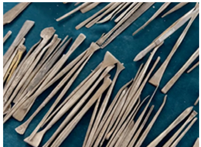
Figure 5. Tools used by Persah Cezayirliyan to shape carton-pierre motifs. Gazete Duvar .
